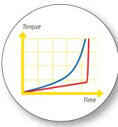
The red line indicates the steep increase in torque with hard applications, e.g. in metal.
