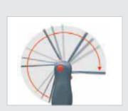
The 270° stop limit when working on applications with higher safety requirements puts an end to trapped fingers.
