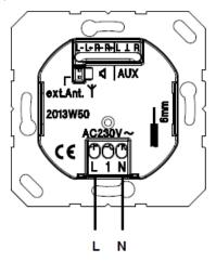
It is not allowed to use the terminals to loop through wires.
