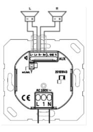
In the case of manual switch-over to mono operation (2 x mono), the radio can also be used with just one loudspeaker.
