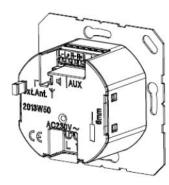
To connect the cord aerial, remove the jumper. Make sure to store the jumper for later use of the radio without cord aerial.
