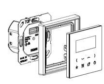
The flush-mounted power supply unit contains the connections for the mains voltage, loudspeaker and possibly the extension.
