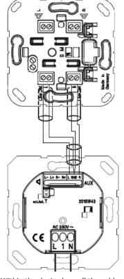
Within the device box, all the cables carrying low voltages (including the optional cord aerial) must have an insulating hose, in
