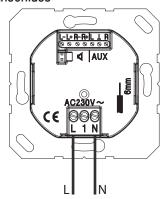
The Bluetooth Connect requires a permanent mains connection. A loopthrough via the connecting terminals is not permitted.
