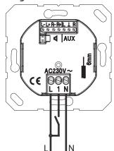
The extension unit connection (1) is used to switch the Bluetooth Connect on/off via switches, e.g. together with the light. The extension unit input may only be operated on the same phase.
