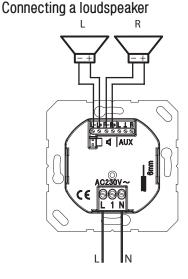
The device is intended for operation with one or two loudspeaker modules LSM.... The connection cable can be up to 5 m long.
