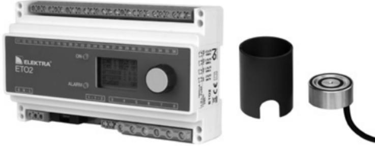
ELEKTRA ETOG2 controller – max. load up to 3x16 A. For applications in extended heating systems. As standard, equipped with one temperature and moisture sensor and an installation tube. Additional temperature and moisture sensor can be connected to this controller, which will enable protection of two outdoor areas. Enables control of two independent zones, e.g. garage driveway and gutters, with one controller.
