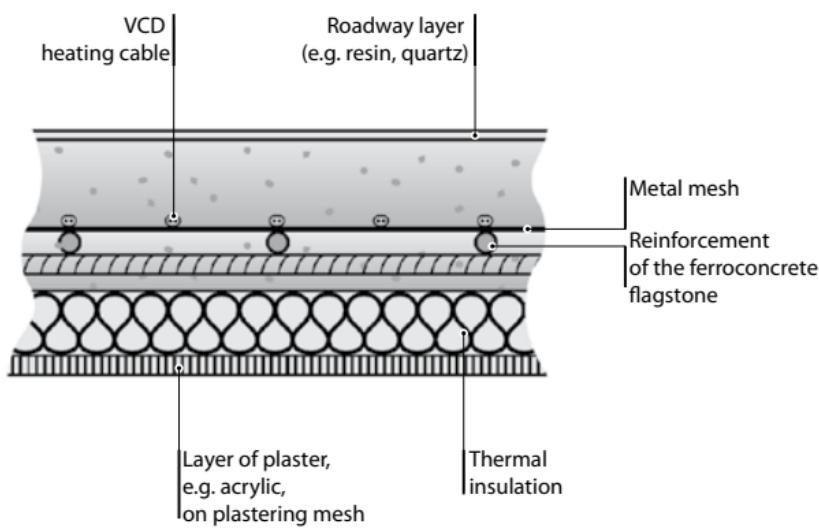
Cross section of a suspended loading ramp
