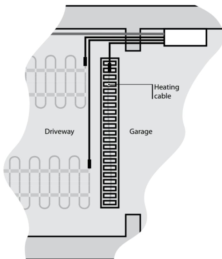
Linear drainage heating
