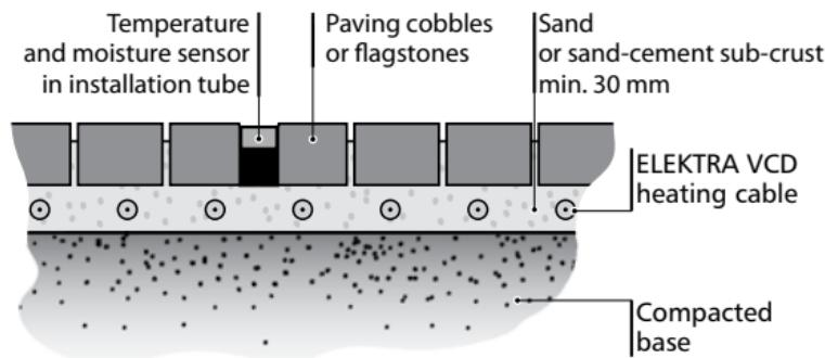
Cross section of pavement or driveway made from flagstones or paving cobbles
