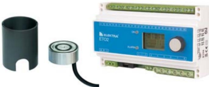
ELEKTRA ETOG2 controller – max. load up to 3x16 A. For applications in extended heating systems. As standard, equipped with one temperature and moisture sensor and an installation tube. Additional temperature and moisture sensor can be connected to this controller, which will enable protection of two outdoor areas. Enables control of two independent zones, e.g. garage driveway and gutters, with one controller.
