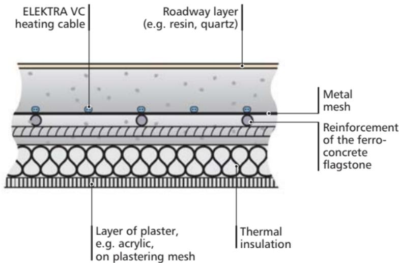
Cross section of a suspended loading ramp
