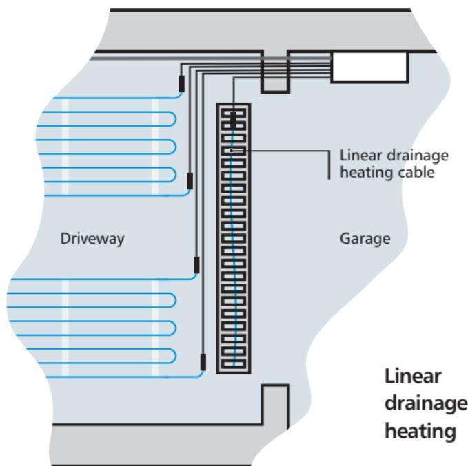
It is also necessary to heat the floor drain (drainage) in order to ensure the outflow of water originating from snow melting. For this, use ELEKTRA SelfTec®PRO 33 self-regulating cable. Place the cable at the through bottom, enter the cable's end into the drainage down to 0.5 m – 1.0 m deep.
