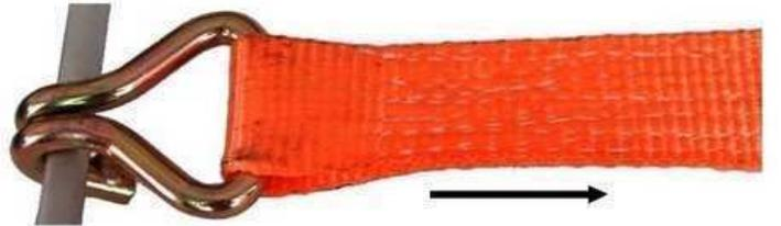
**5** Pull up to collect all the excess belt
