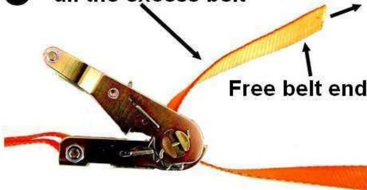
**6** Operate the lever ratchet for tensioning of the belt
