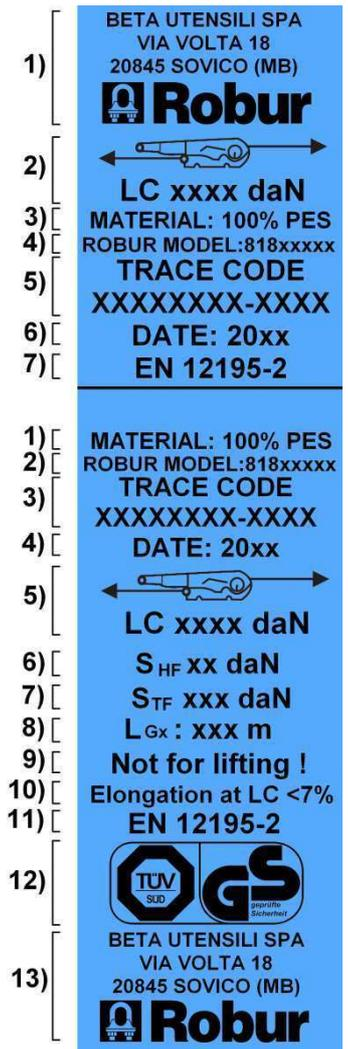
The blue colour of the label immediately identifies the material the strap is made of, namely 100% PES (polyester).
